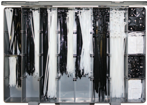
BLACK & WHITE WIRE TIES KIT Part Number KIT-TIES Popular 4", 5", 7", 8", and 11" cable ties with tensile strengths of 18 to 120 pounds. 3/4" and 1" adhesive mounts. 900 pieces. Drawer satchel.
