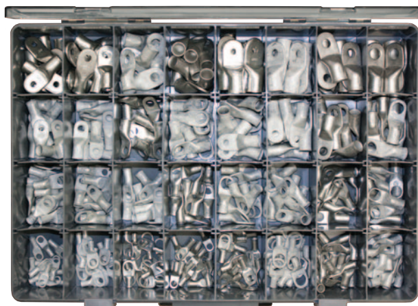
PLATED LUG KIT Part Number KIT-BCL Heavy-duty closed-end plated copper eyelet lugs. 1/4", 3/16", 5/16" and 1/2" eyelets in 8 to 4/0 gauges. 355 pieces. Drawer satchel.
