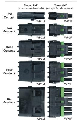
**Weather Pack Locking Connectors** seal out moisture and dirt. These one- to six-contact nylon connectors are rated -40°F to 257°F, up to 16 volts DC and 20 amps. Hinge lock assembly. Self-lubricating silicone body seal reduces engagement force. Silicone cable seals must be used with the tin plated brass terminals. The cavity plug fills unused pin locations. Terminals and seals sold in quantities of 100.
